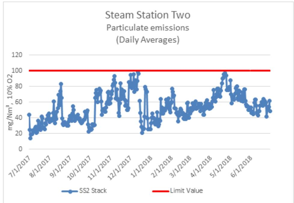
As indicated within the December 2017 monthly report, a deviation was experienced on Steam Station 2 on 14 December 2017 which was associated with an instrument error and an upset condition. The slightly elevated concentration was flagged and removed for reporting purposes as it was associated with abnormal conditions.
