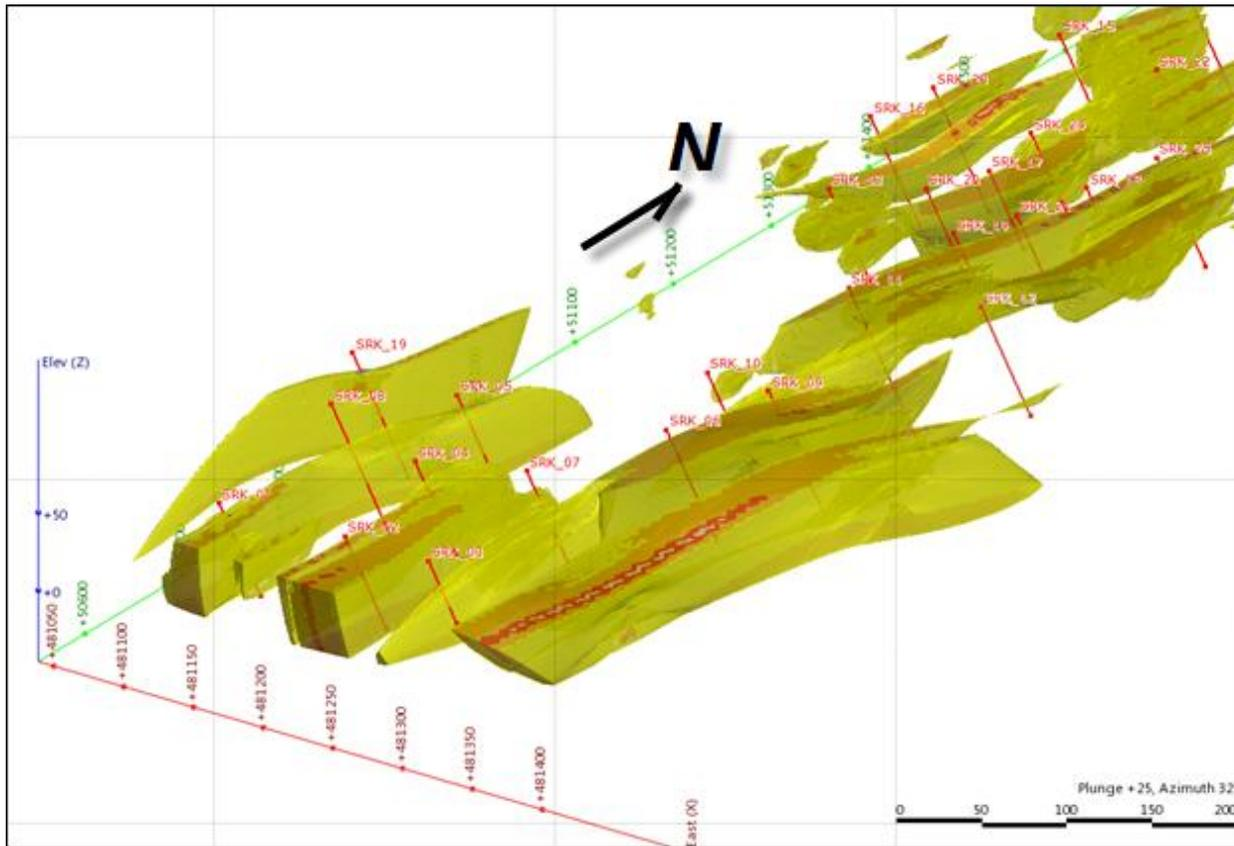
**Resistivity survey - NNE trending, steeply dipping series of zones of high conductivity ( $>0.21$  S/m)**
