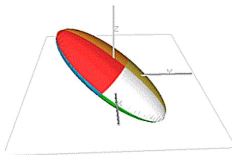
**Figure 1: Oriented search ellipsoid (Source: Copyright © Datamine 2016).**
