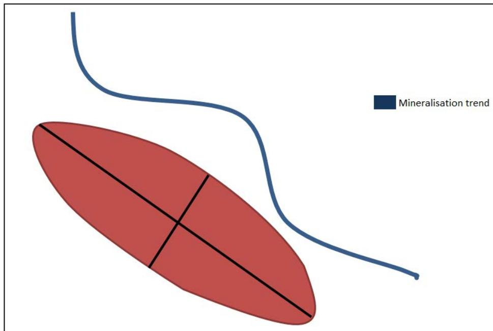
**Figure 2: Search ellipsoid oriented along most continuous direction of mineralisation.**
