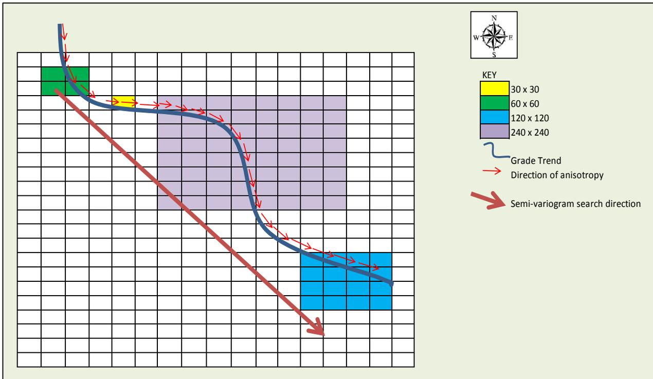
**Figure 19: Diagrammatic representation showing relationship between block sizes, “resolution of Dynamic Anisotropy” and localised directions.**
