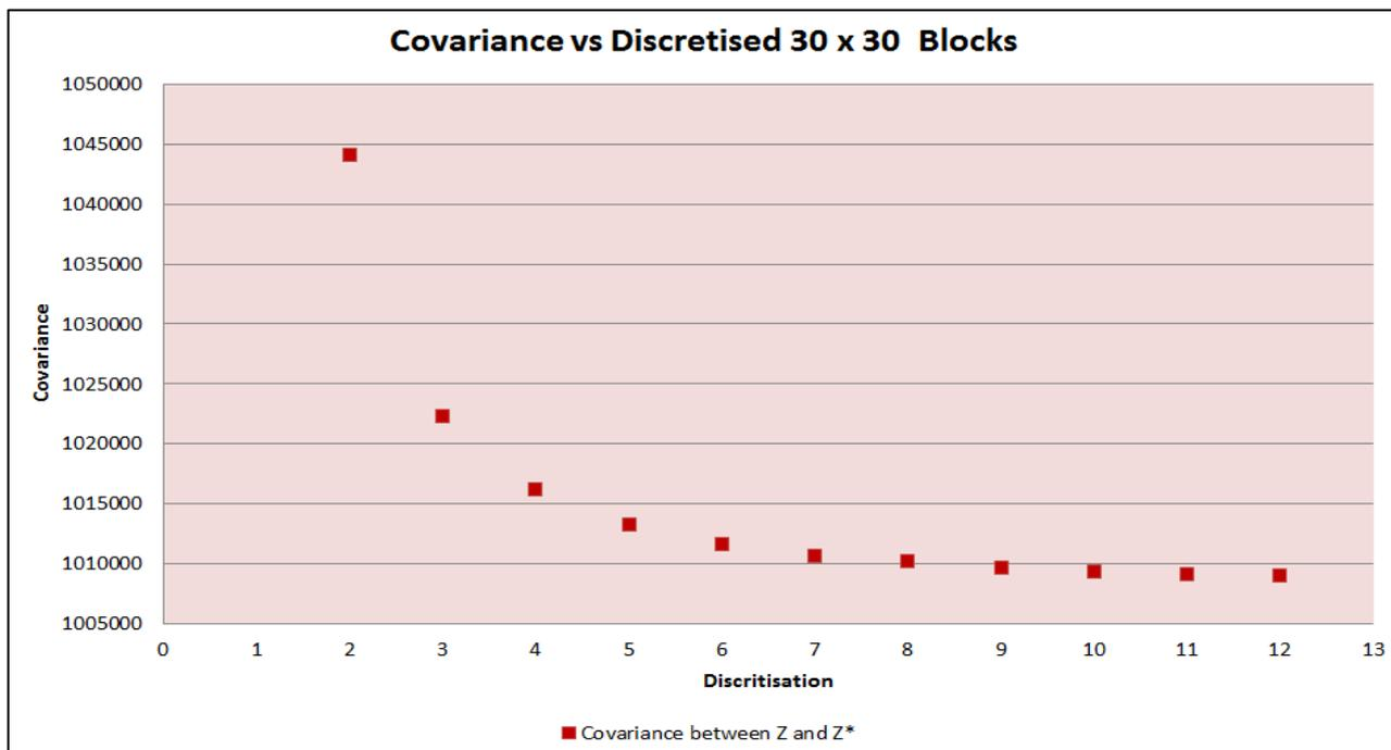
**Figure 13: Graph showing sensitivity of covariance to block discretization.**
