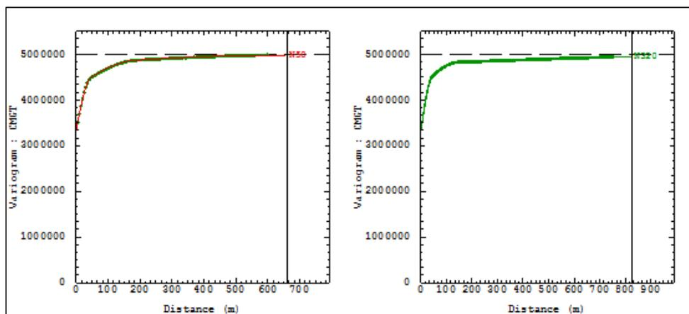
**Figure 11: Back-transformed Cm.g/t experimental and model variogram for short (N50, left) and long (N140, right) directions**
