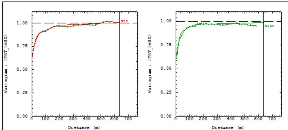
**Figure 10: Variogram models for short (N50, left) and long (N140, right) directions**
