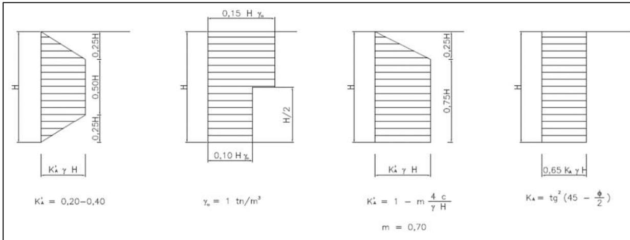
Figure 4. Code diagrams of minimum design earth pressures for strutted excavations
