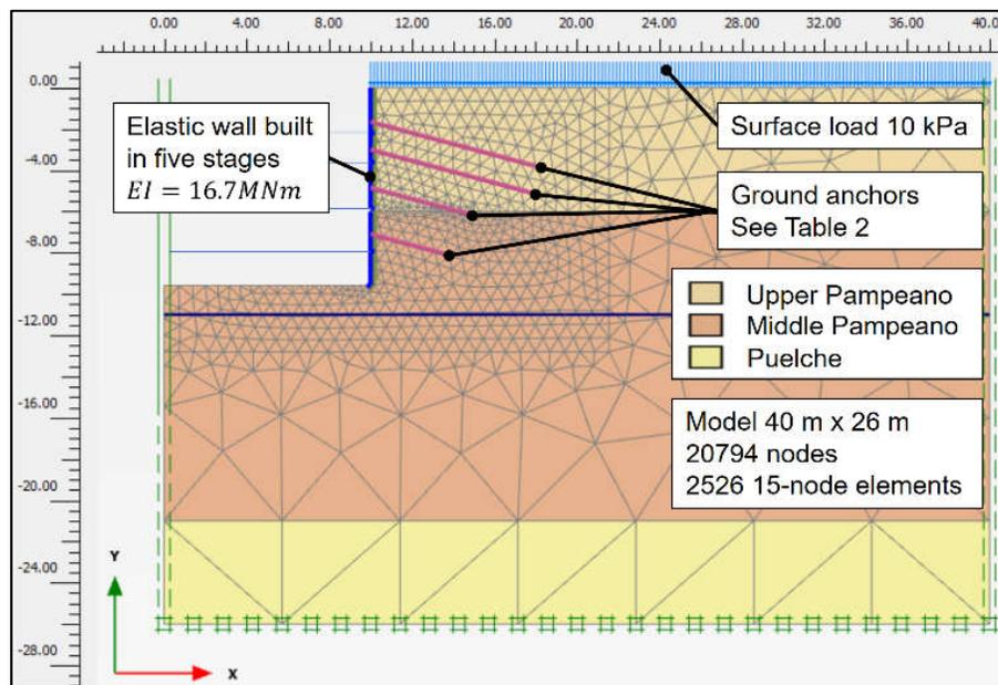
Figure 16. Geometry and finite element mesh.
