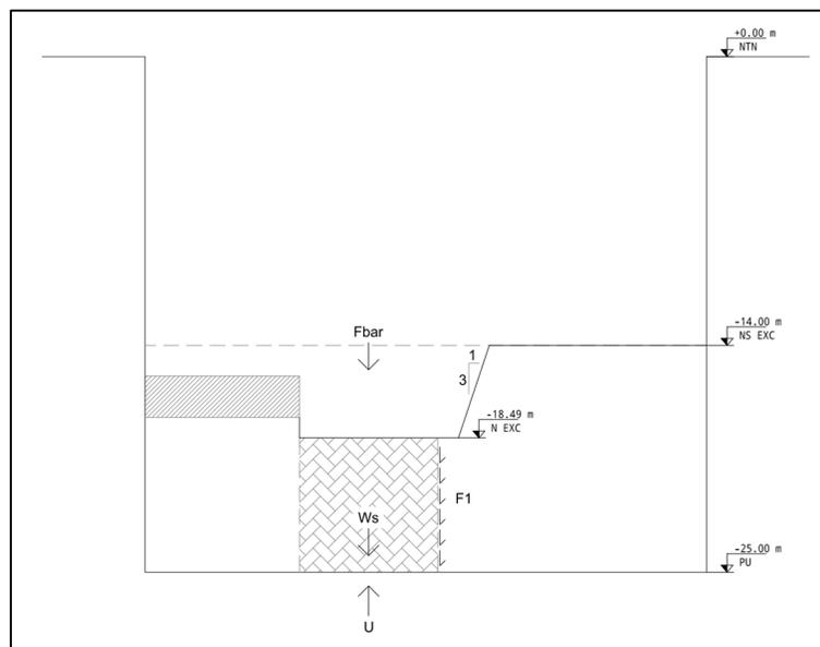
Figure 12. Forces acting on the soil plug in region 1-B.
