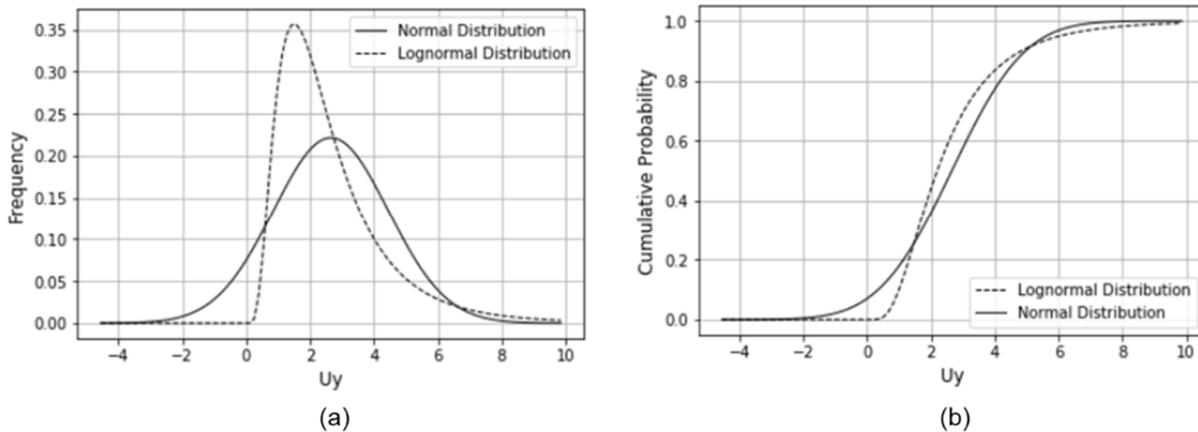
Figure 17. Distribution of probability (a) and cumulative probability (b) of the vertical displacement  $U_y$  for uncorrelated cohesion and friction angle using PEM (Ledesma et al 2019).
