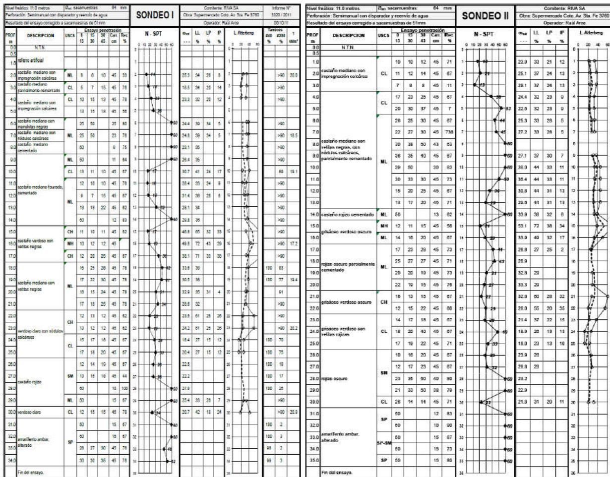
Figure 3. Two typical boreholes in Buenos Aires city center (Laría et al 2015).
