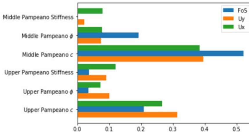
Figure 18. Sensitivity score of input parameters for different target functions:  $FoS$ ,  $U_y$  and  $U_x$ .
