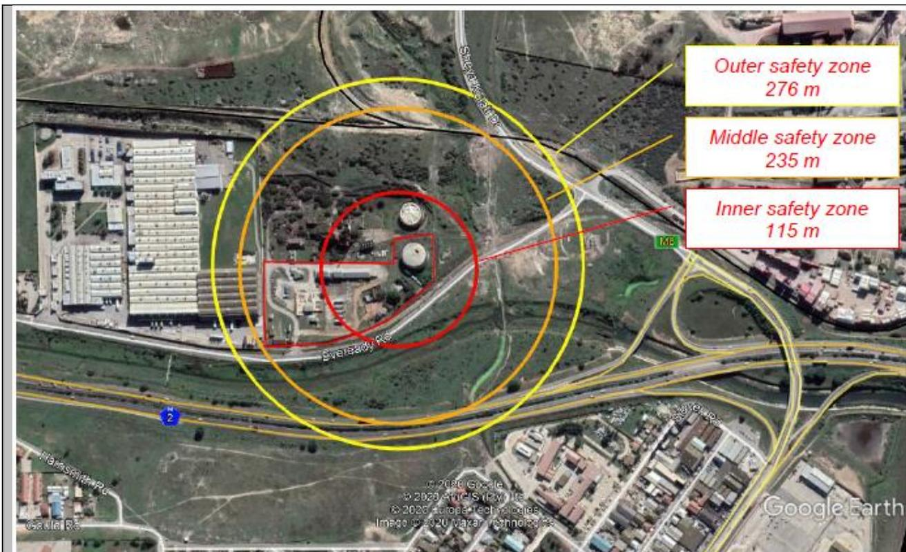
**Figure 1: Safety Risk isopleth map for the site, including the new proposed 400 m3 tank**
