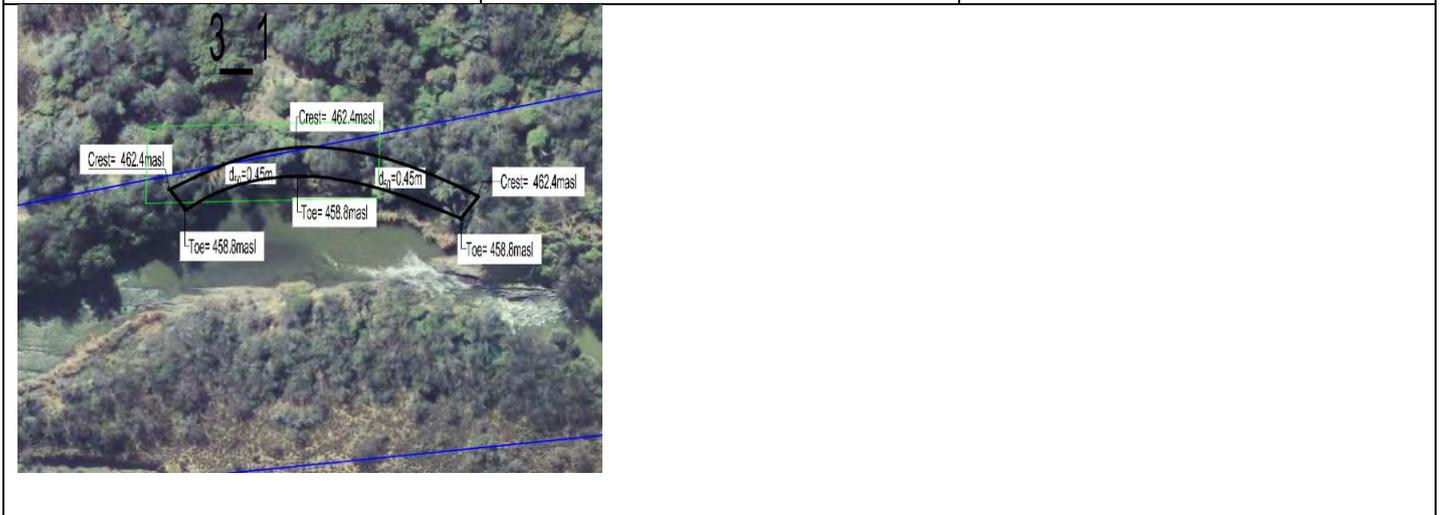
**Zone 3\_2** Flow in this area is in a wide floodplain crossing the servitude and protection is not viable.
