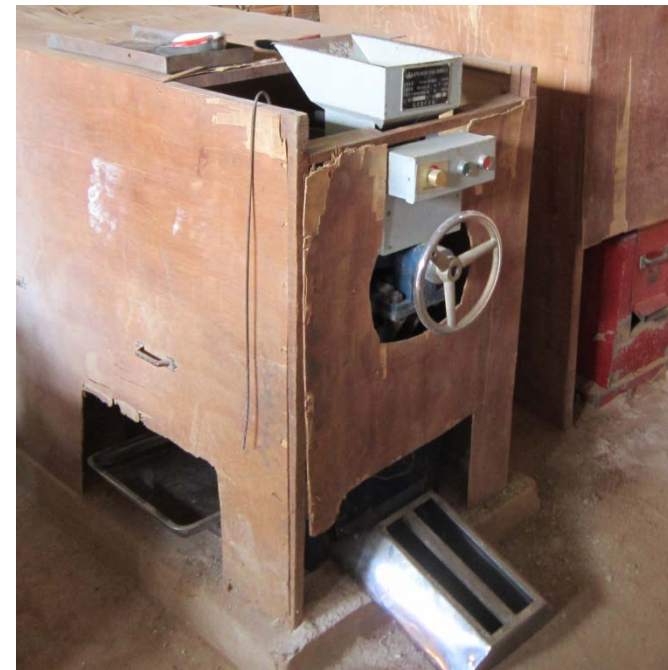
Sample crushing equipment, poorly maintained and not cleaned
