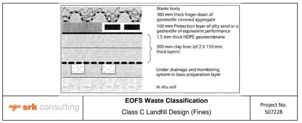
Figure 5-2: Class C Inert Landfill Barrier Design (GN 636)
