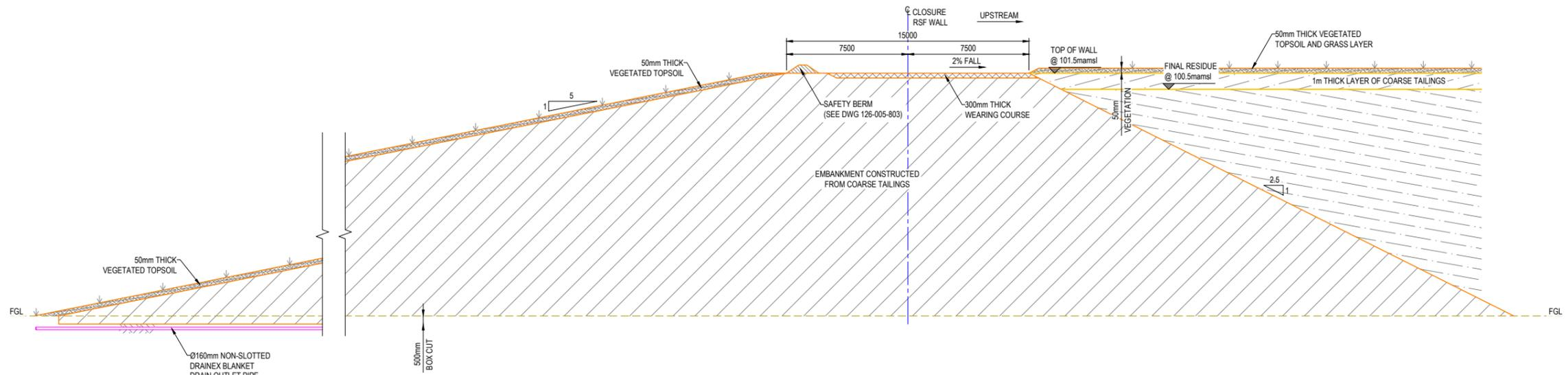
TYPICAL SECTION THROUGH CLOSURE RESIDUE STORAGE FACILITY WALL
