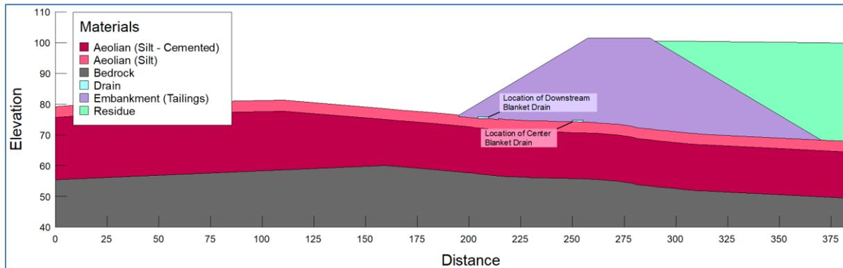
FIGURE 8-3: OPERATIONAL PHASE – RESIDUE AT MAXIMUM CAPACITY
