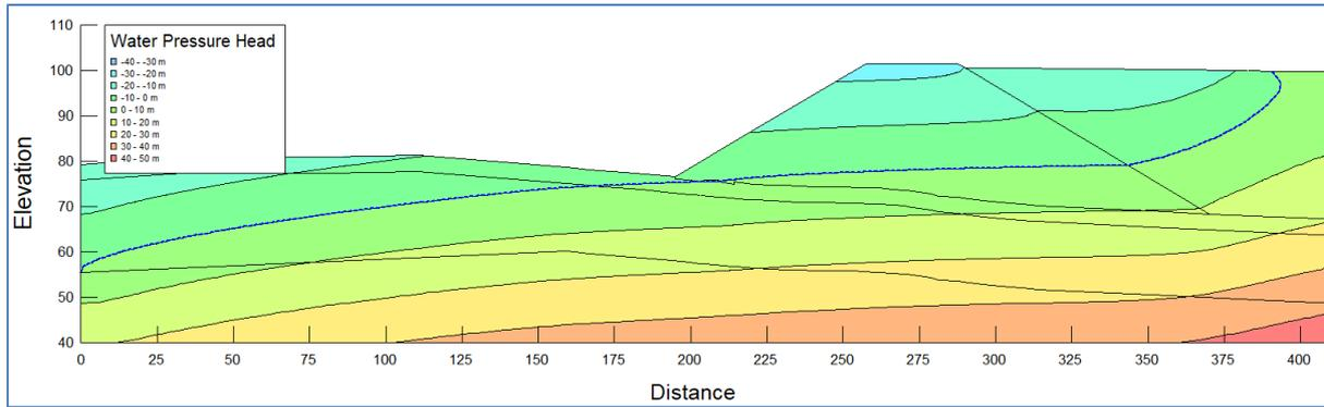
**FIGURE 9-3: OPERATIONAL PHASE AT CAPACITY, SEEPAGE ASSESSMENT OF THE RD WITH AN ACTIVE DOWNSTREAM BLANKET DRAIN**
