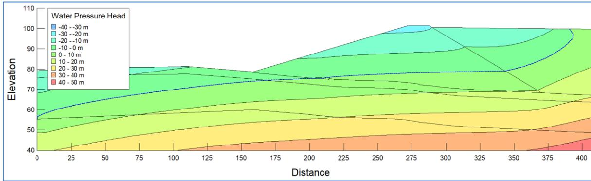
**FIGURE 9-6: CLOSURE PHASE AT CAPACITY, SEEPAGE ASSESSMENT OF THE RD WITH AN ACTIVE DOWNSTREAM BLANKET DRAIN**
