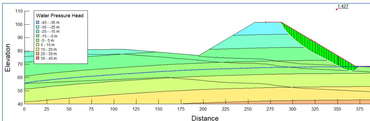
FIGURE 11-1: UPSTREAM FACE OF THE OPERATIONAL PHASE WITH INITIAL RESIDUE DEPOSITION (SEISMIC LOADING)
