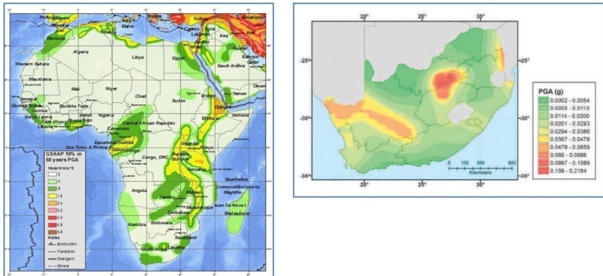
FIGURE 10-2: PEAK GROUND ACCELERATION (GHSAP (LEFT) AND COUNCIL OF GEOSCIENCE (RIGHT)).
