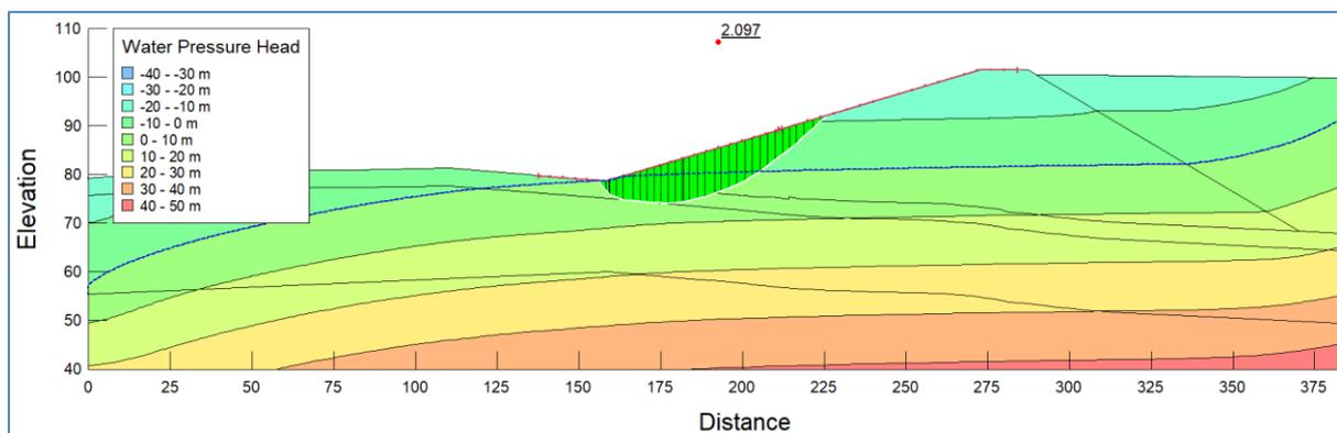
FIGURE 11-3: DOWNSTREAM FACE OF THE CLOSURE PHASE WITH RESIDUE AT MAXIMUM CAPACITY (SEISMIC LOADING)
