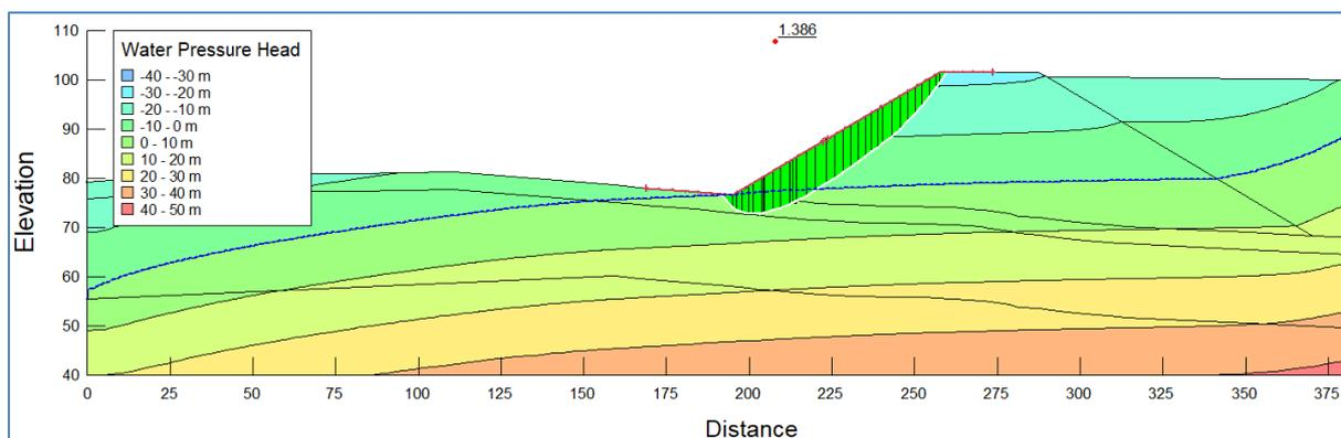
**FIGURE 11-2: DOWNSTREAM FACE OF THE OPERATIONAL PHASE WITH RESIDUE AT MAXIMUM CAPACITY (SEISMIC LOADING)**
