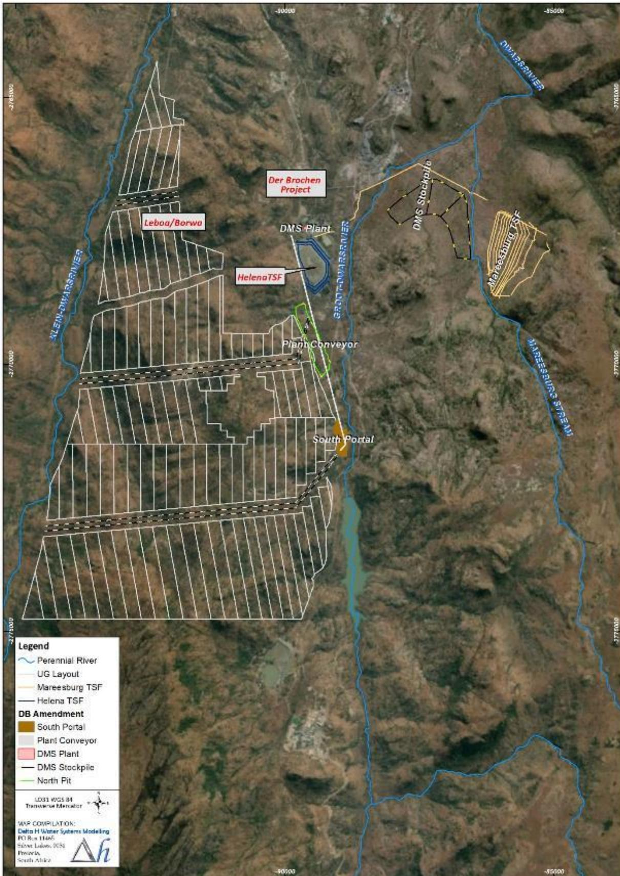
Figure 1-1: Der Brochen Mine's Expansion Project – Infrastructure layout.
