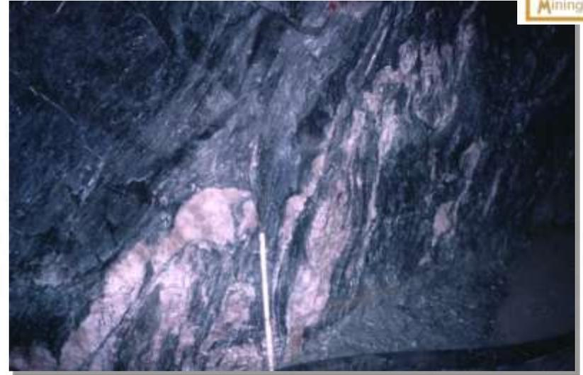
Boudinaged and isoclinally folded quartz vein.
