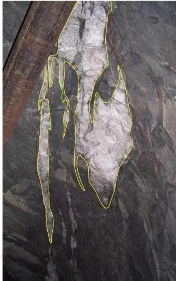
Boudinaged and isoclinally folded quartz vein.
