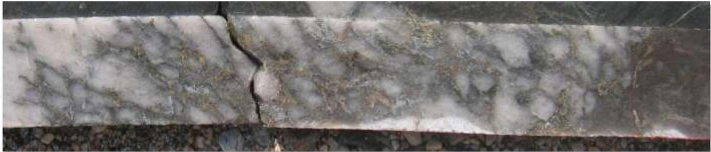
Pyrrhotite-pyrite-chalcopyrite extensional vein array
