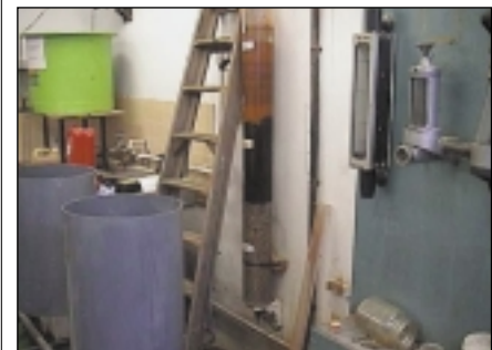
Figure 3: Laboratory reconstruction of the Pelenna SAPS
